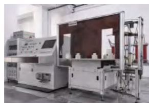
Power Frequency Withstand Voltage Test Equipment
